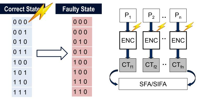
Example: Consider a stuck-at-0 fault at the LSB bit of the intermediate state. The faulty state can only assume even values.
