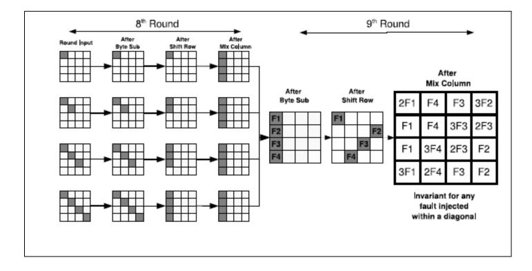
Faults induced in Diagonal D<sub>0</sub> at the input of 8<sup>th</sup> round AES are all equivalent.
