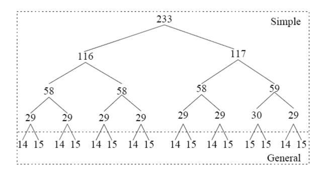
The multiplier operates on 233 bit inputs and gives a 465 bit outputs.
